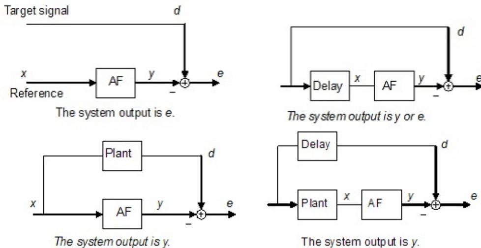
Fig. 4: Typical applications of adaptive filters. Top-left: interference cancellation, top-right: prediction, bottom-left: identification, and bottom-right: inverse modeling.
