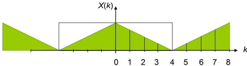
Fig. 2: Spectrum and the frequency index in the 8-point DFT.
